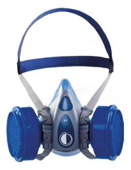
The RPA-DE half mask with two FRPA P2 particle filters is used in severe production environments at high/low temperatures, high humidity, and in prolonged heavy-duty operations with a working air dust content of up to 1,000 mg/m³.
